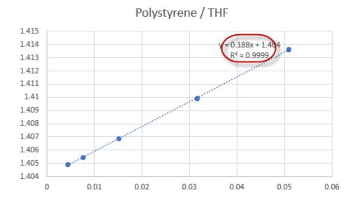
In fact, the Rudolph x57 Series Refractometer has a built-in feature to calculate dn/dC. Using the Custom Scales feature and inputting only two points gives the following result:
