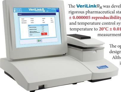
The **VeriLinkR**<sub>X</sub> was developed by Rudolph using technology predicated on rigorous pharmaceutical standards such as USP<831>. To meet the **verifiable**  $\pm$  **0.000005 reproducibility** the **VeriLinkR**<sub>X</sub> has a highly stable measurment and temperature control system allowing the **VeriLinkR**<sub>X</sub> to stabilize the sample temperature to **20**°C  $\pm$  **0.01**°C, before measurement thereby elliminating measurment and temperature errors.
