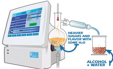
After distillation, the water and alcohol are separated from the sugars and flavors. Once this process is finished the separated alcohol and water can be measured in a stand alone density meter.
